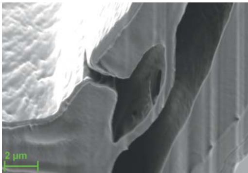
Figure 8.2: Bordered pit in the cell wall of a soft wood tracheid, connected to an interstice between the cells (2 kV U_{EHT} , 4.7 mm WD, SE2-detector).
