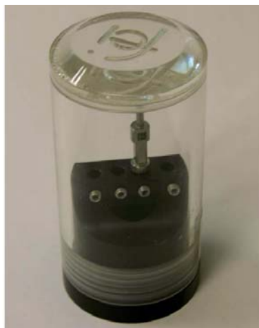
Figure 3.15: A possible transport solution made from an SEM cathode box for FIB processed specimen on IBL holders to ensure a safe transport to DESY. The IBL holders are easily accessible by tweezers and fixed by grub screws. The box should be additionally wrapped in something soft and vibration absorbing for transport.
