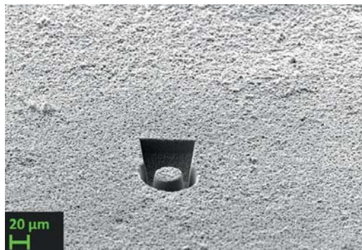
(a) Excavation from the photonic glass (20 kV U_{EHT} , 5 mm WD, SE2-detector)
