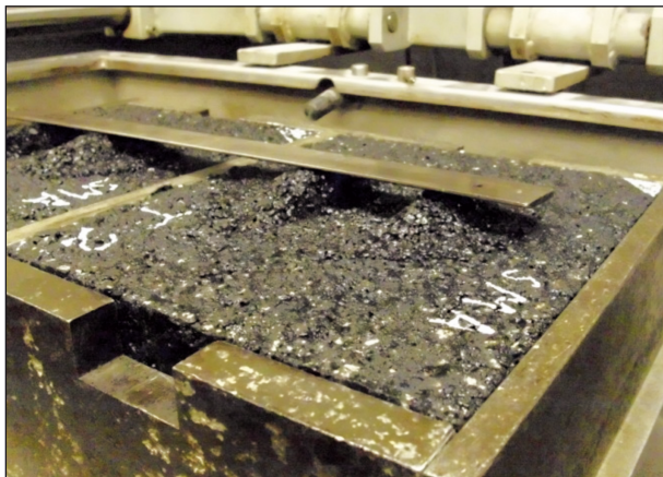
Fig. 1: Test sample filled with repair material in groove formation test
