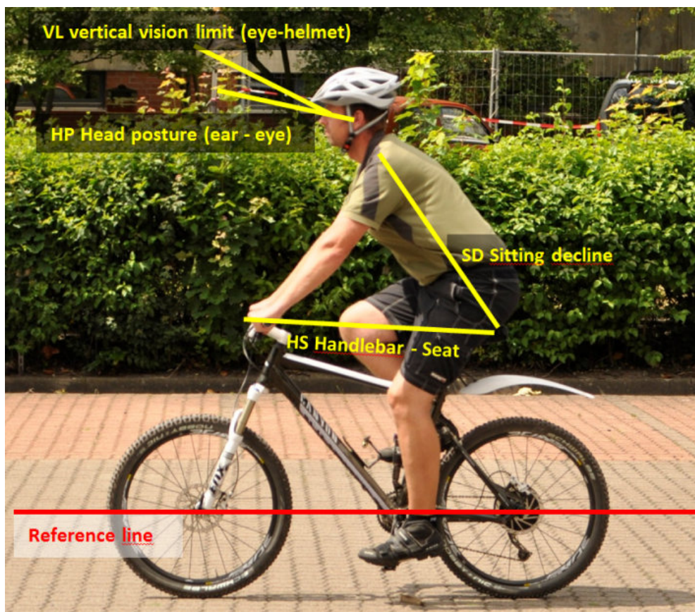
Figure 7: Establishment of angles relevant for seating geometry and vision limits
