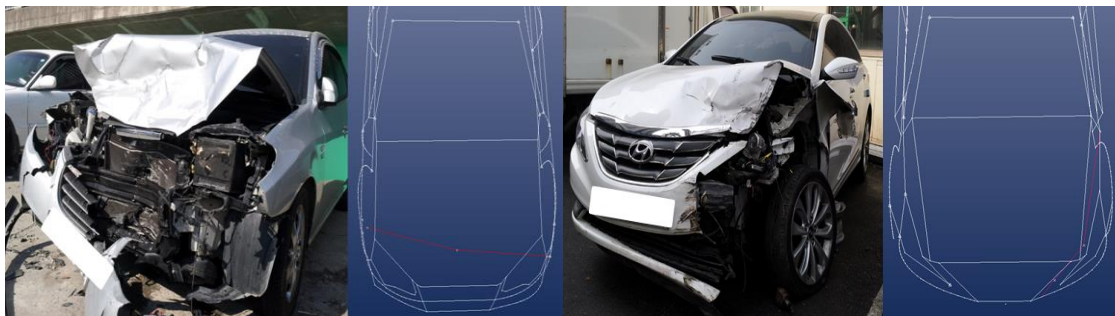
Figure 9. Vehicle deformations calculation using PhotoModeler
