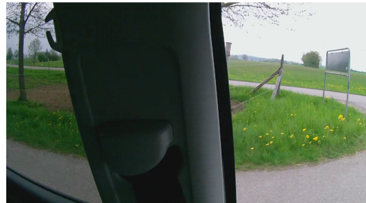
Figure 8: Impact of seat posture on visibility to the sides (compact MPV)
