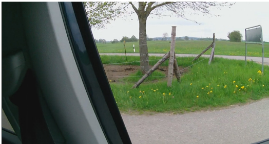
Figure 8: Impact of seat posture on visibility to the sides (compact MPV)
