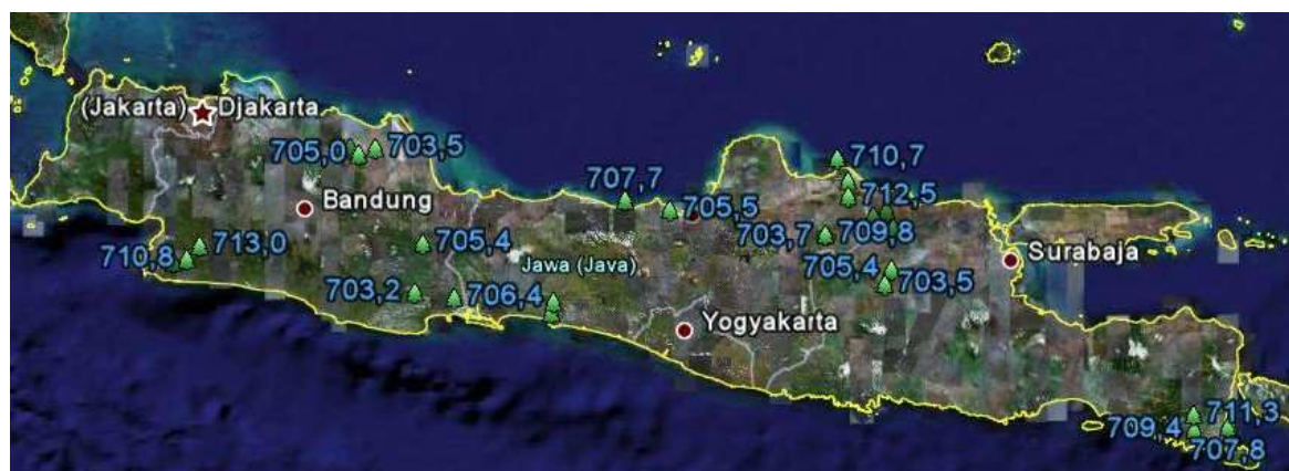
Figure 24: Isotope ratios of strontium ( ^{87}\text{Sr}/^{86}\text{Sr} ) in Java, factored with 1000
