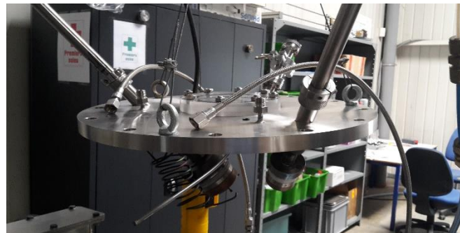
Figure 20: Reactor with Home Concrete Vibrators.
