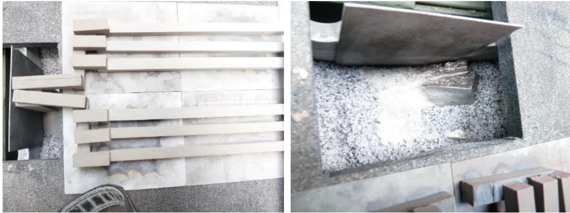
Figure 62: Infiltration circuit with BNi7, before (left) and after treatment (right).
