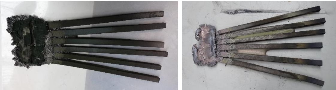
Figure 65: 316L pre-sintered bars infiltrated with BNI7 (left) and with F300 (right).
