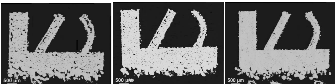
Figure 45: Metallographic cross sections of built test parts with CuNi3Si (95 W – 200 mm/s) Effect of powder layer thickness on porosity (20 µm – 15 µm – 10 µm – respectively 6.6 %, 3.0 % and 1.3 % porosity) for optimal powder size with the CuNi3Si alloy (10-25 µm)
