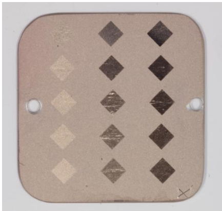
Figure 23: Example of a CuSn sheet after the laser test. The squares were lasered with different laser powers and speeds.
