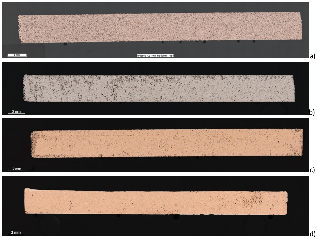
Figure 59: Metallographic investigations on infiltrated Cu parts – a) Pure Cu part as built b) part infiltrated with Silver solder Ag 71,5% - Cu 28,5% c) part infiltrated with Silver solder Ag 70,5% - Cu 27,5% - Zn 2% d) part infiltrated with Silver solder Ag 85% - Cu 15%
