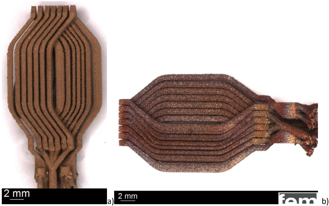
Figure 57: Electric motor coil (design by Unicorn Engineering GmbH) built with LBM a) with CuNi3Si (10-25 \mu\text{m} powder size and 10 \mu\text{m} layers) b) with Ti coated Cu powder (10-45 \mu\text{m} and 20 \mu\text{m} layers)
