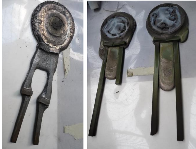
Figure 67: Bars printed with Cr coated 316L powder infiltrated with BNi7 (left) and F300 (right)
