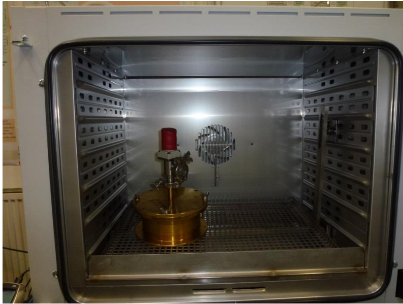
Fig. 3.2 Isopiestic vessel inside an oven
