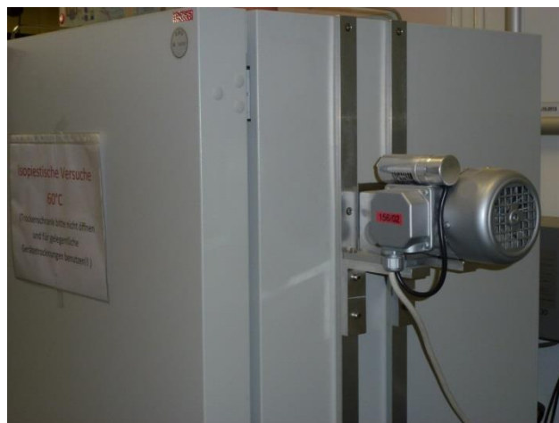
Fig. 3.3 This picture shows a motor fixed at the outside of an oven to exert a gentle rocking motion to the board on which the isopiestic vessels rest
