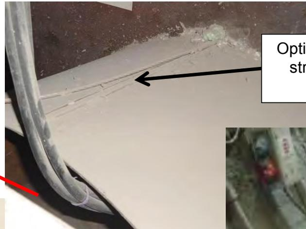
Optical fiber for distributed strain and temperature measurements
