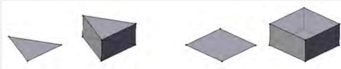
Extrusion of a triangle and a quadrilateral.
