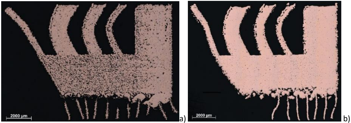
Figure 93: Metallographic examination of the test part made of PureCu (process parameter 380 W - 600 mm/s - track spacing = 0.065 mm) – a) PureCu - porosity 15.9 % / b) PureCu + W - porosity 0.9 %
