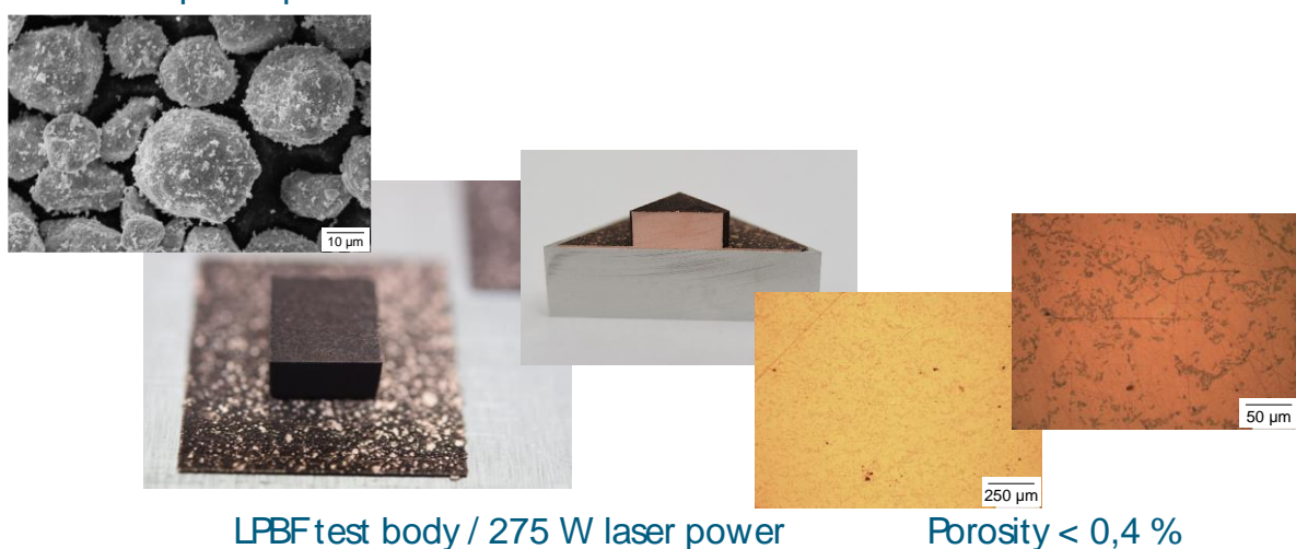
Figure 115: Test body and microsection from a manufactured cube by using mixed/milled Cu with 3 vol.-% W.
