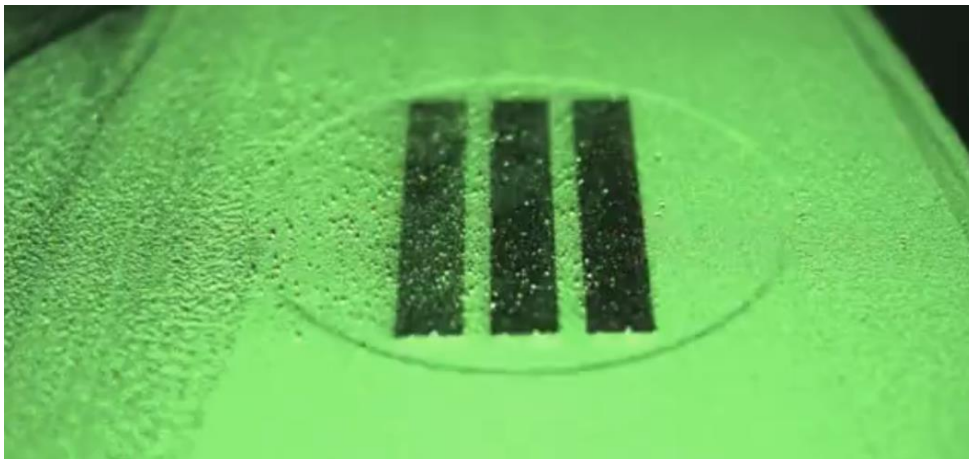
Figure 105: LBM process - snapshot after the laser exposure - smoulder deposition on the parts increasing from right to left (according to the gas flow direction)
