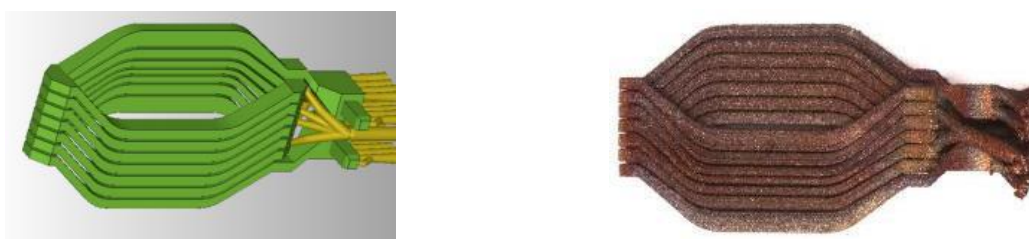
Figure 6: Coil for highly efficient electric motors (Design by Unicorn Engineering GmbH): (left) CAD Design / (right) Part additively manufactured by LBM employing Ti-coated powder.
