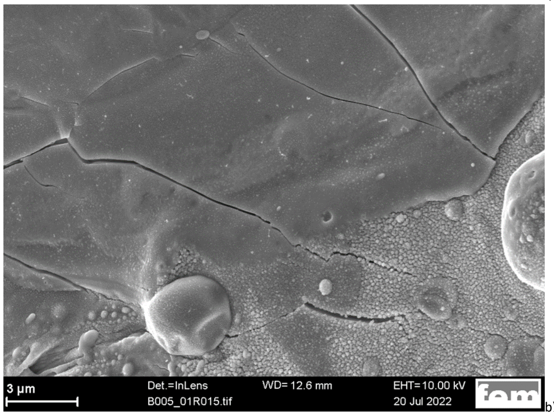
Figure 112: SEM investigation of a lack of fusion defect in the fractured surface of a CuNiSiCr + Nb sample a) overview b) detail of insufficient wetting of the smoulder covered area
