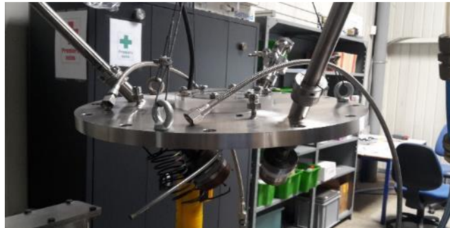
Figure 37: Reactor with Home Concrete Vibrators.
