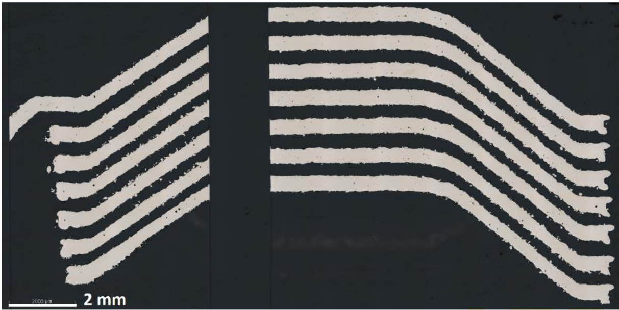
Figure 97: Metallographic examination of the demonstrator (coil for electric motor). CuNiSiCr alloy.
