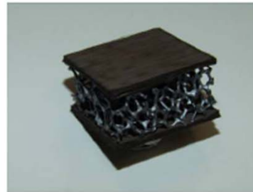
CMC/Foam sandwich progress (EADS-IW, C. Wilhelmi)
