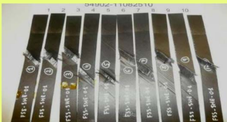
Shear failure on M40J/M18 MD specimens at 180°C
