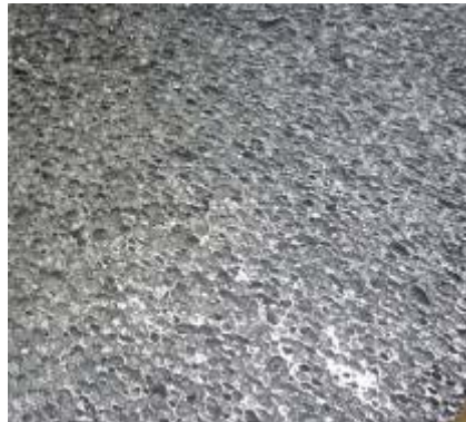
Metallic foam/ hard ALCaTi alloy 250 kg/m 3
