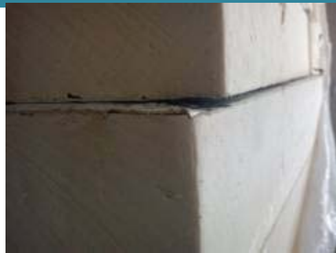
Soft PU foam with Al coating ; 30-40 kg/m 3
