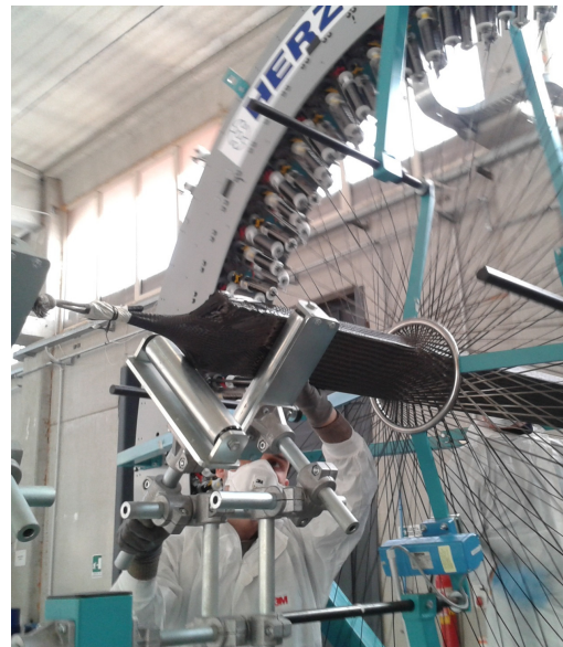
Fig. 10: Braiding on squared mandrel
