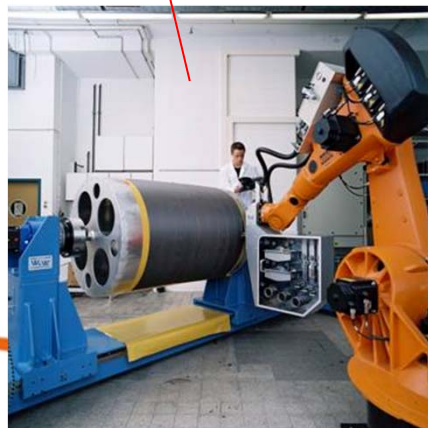
green body (prepregs) winding and lamination
