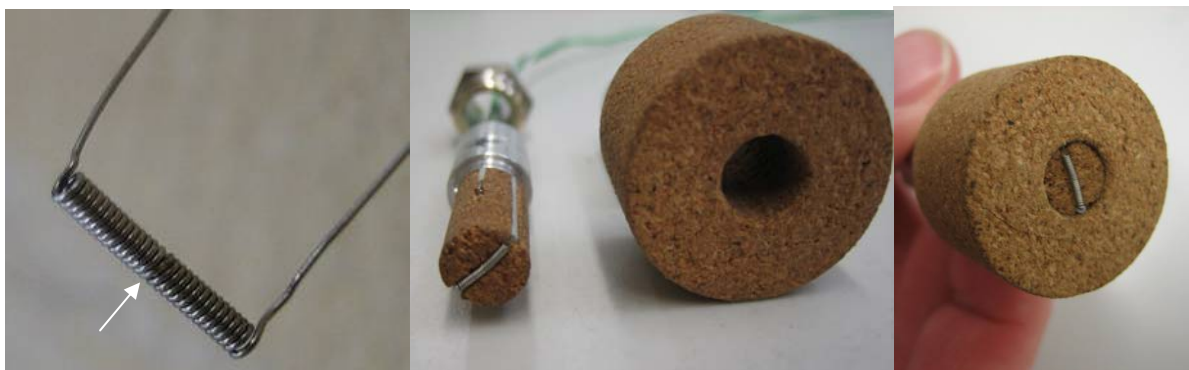
Fig. 9. Wound Thermocouple and press fit plug
