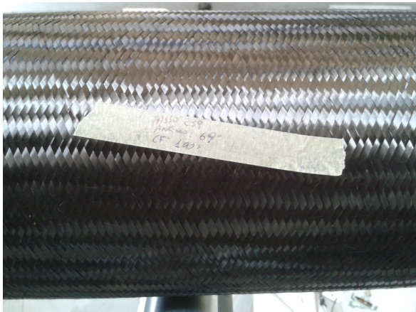
Fig. 9 Carbon fibers braiding at 60^\circ on cylindrical mandrel
