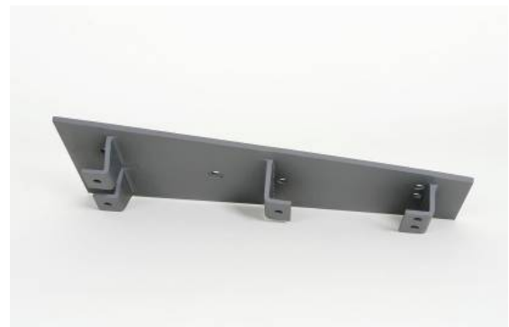
Fig. 7: C/SiC Ceramic Experiment Design & Experiment as manufactured and integrated on SH II
