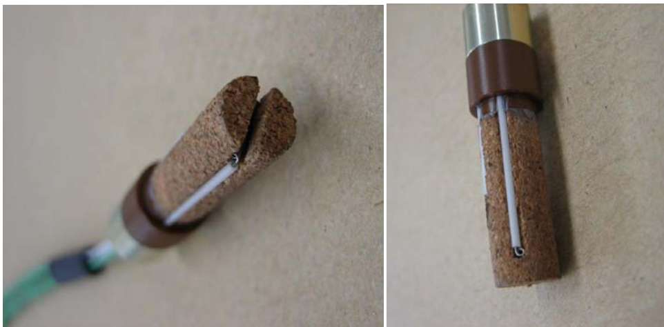
Fig. 8. Comparative performance samples: grooved plug (left) and drilled plug (right)
