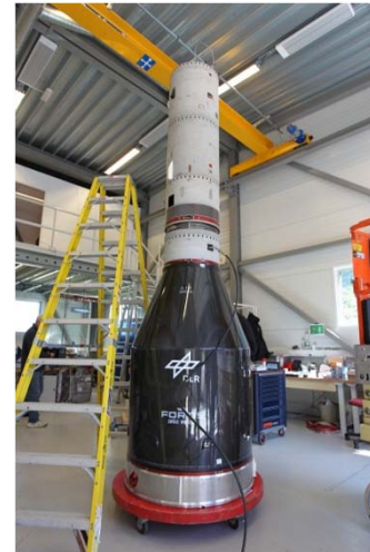
CFRP Fairing with integrated ablative TPS
