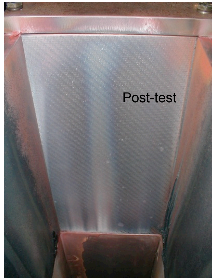
Discoloration due to melting of carbon steel fixturing
