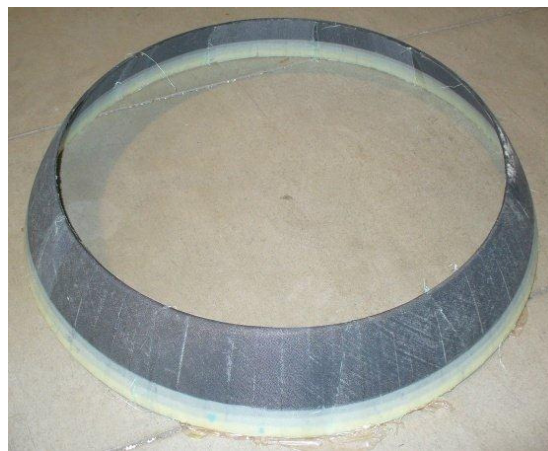
Fig. 6: 1st prototype of hybrid composite spherical reinforcement shims at Z23 scale
