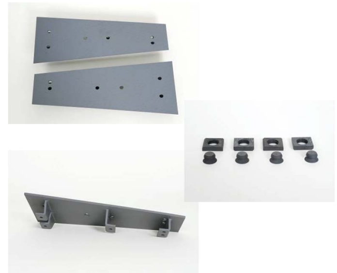
after machining & coating incl. fixation elements
