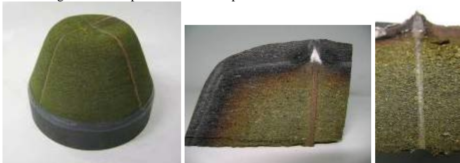
Figure 6: ASTERM TPS before and after Scirocco arc jet test
