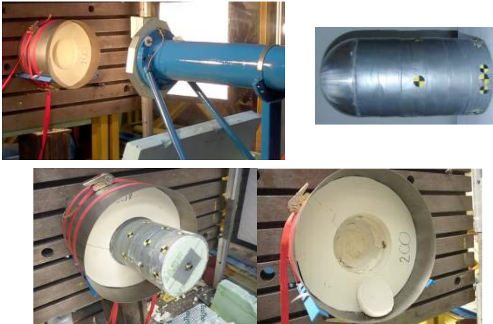
Figure 15: Cannon and 5.5 kg bullet (top) – Impacted foam block (bottom)
