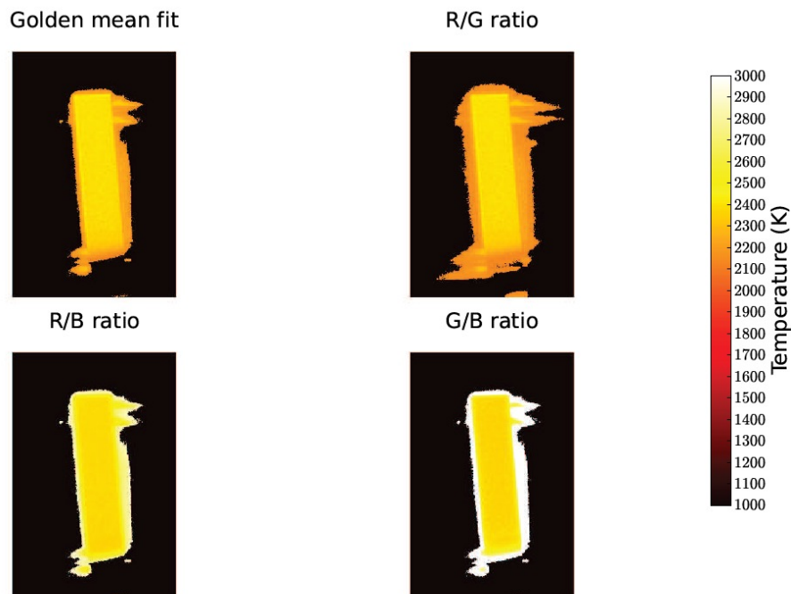
Figure 2. Temperature distribution across the tungsten ribbon, set at 2400 K, as processed by the three possible RGB ratio sets, and the optimized combination.
