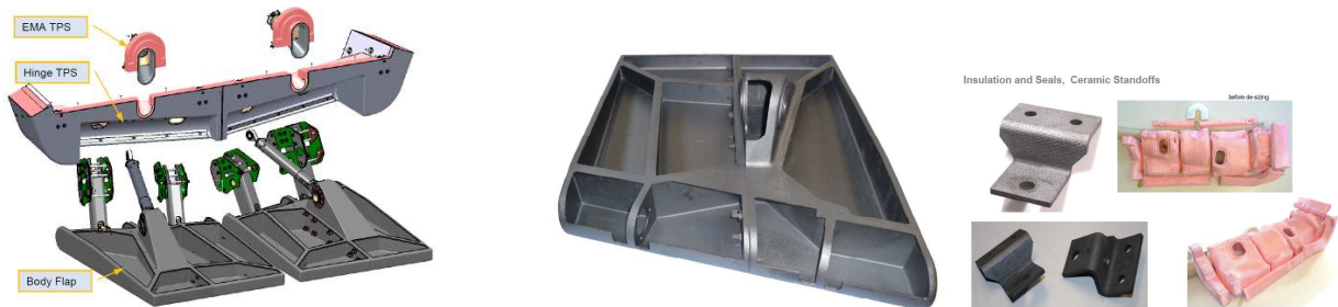
Figure 5. Body Flap Assembly design (left side) and QM manufactured parts (right side)
