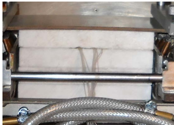
Fig.16. Assemblage made from two specimens A and B into experimental module.
