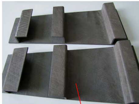
green body (prepregs) winding and lamination
