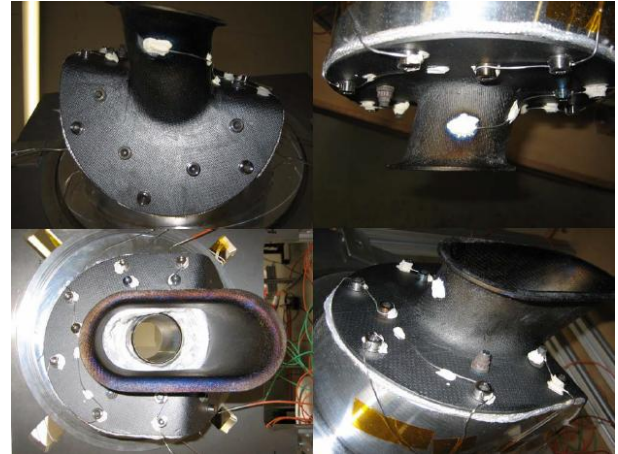
Fig. 20: CMC Adapter after second Preconditioning Test
