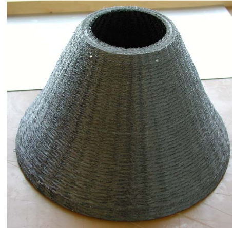
Exemplary image of braided structures for the Fuel-Cooled-Ceramic-Nozzle (FCCN) in Dual-Bell contour
