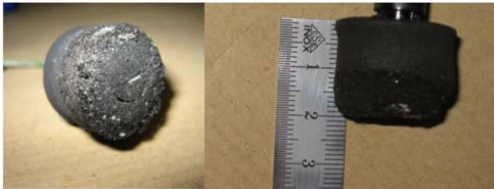
Fig. 11. Ablation pattern of drilled thermocouple
