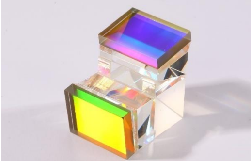
Fig. 6: Picture of the assembled Spatial Heterodyne Spectrometer (SHS). The yellow and blue surfaces are the gratings.
