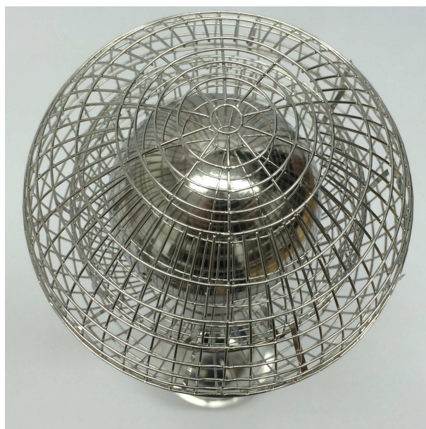
Figure 1. Meteor Smoke Particle Detector with its central spherical electrode (26 mm radius) shielded by two concentric and electrically biased grids (35 mm and 45 mm radius).
