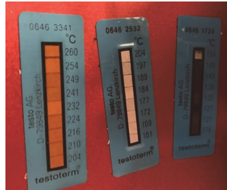
Figure 9. Temperature strips of the uppermost module (Umbilical Module) at 0° after flight. Black color indicates maximum hull temperature
