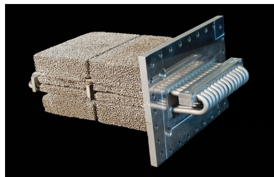
Figure 10. Metallic foams set-up: system brazed on PHP
