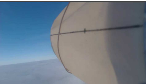
Figure 14. Compressed antenna during decent caused by increasing air pressure due to closed venting valve
