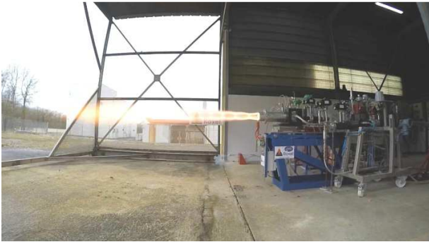
Figure 6: fire test of MLE5K-1sa LOX/Ethanol
