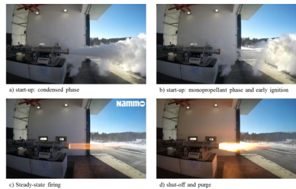
Figure 8: FLPP-UM-016-HRE during the various stage of the firing
