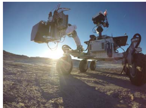
Fig. 8: MESR rover deploying mini-corer and microscope
