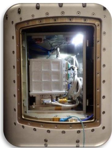
Figure 7. XRMON-DIFF 2 Module with late-access hatch open and DIVA installed.
