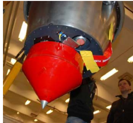
Figure 10. Flight integration of SHARK, mounted on the MAXUS 8 re-entry cone at Esrange Space Center.
