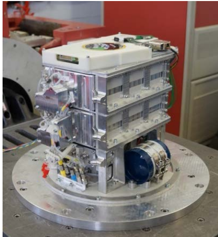
Figure 2. "CEMIOS" flight hardware in ground based test configuration.
