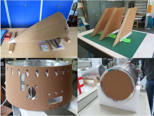
Figure 9. NORCOAT® LIÈGE HPK FI applied on various primary and secondary sounding rocket structures.
