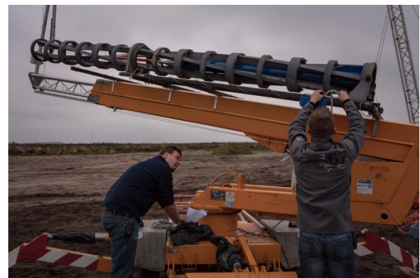
Figure 2. The preparation of the DART system in combination with the T-Minus Engineering multi-rail mobile launcher
