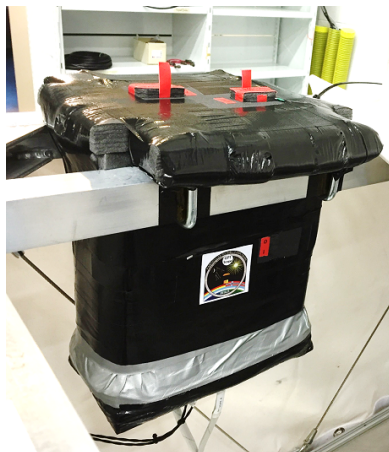
Figure 3. CPT-SCOPE mounted inside the BEXUS 20 gondola. The black material is the thermal insulation and the red labelled places are access points. Gaffer tape was used to keep the insulation in place.
