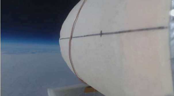
Figure 13. Lid is banging against the rigidized antenna during descent
