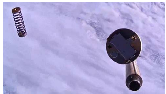
Figure 15. SUPERMAX (middle right ) released from MAXUS payload, after motor (lower right) separation. Also in picture: one of the three separation spring (left).
