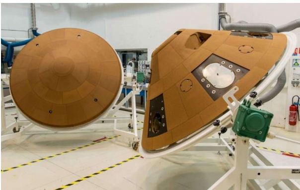
Figure 2. NORCOAT® LIÈGE HPK FI on the Mars re-entry capsule Schiaparelli; source: ESA.
