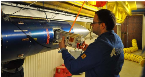
Figure 3. Late access insertion: The rocket was loaded with the living cells through the late access hatch shortly before launch. This assured best possible biological material for the experiments.
