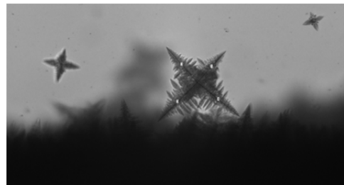
Figure 8.b Equiaxed dendritic growth
