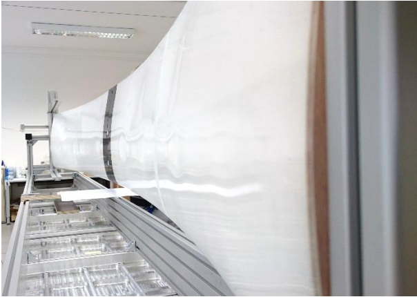
Figure 10: Structural test of ELAHA 10 wing segment
