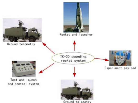
Figure 16. The exploration system of TK-30/TK-32
