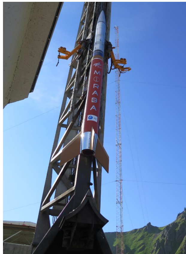
Figure 1. IMPROVED MALEMUTE (IM) vehicle with cork based TPS on fin and motor adapter assemblies.
