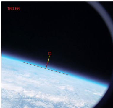
Fig. 10: Scene in the atmosphere at 83.4 km instrument altitude. The red rectangle shows the spectrometer field of view and the yellow line represents the altitude range from 60 km to 120 km.
