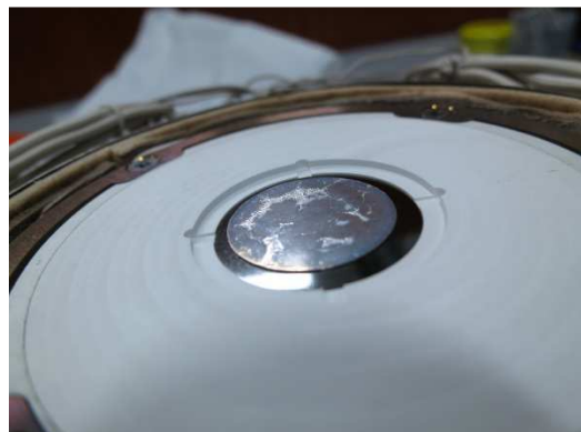
Figure 4. Sample holder and the flight sample, photo was taken after payload retrieval
