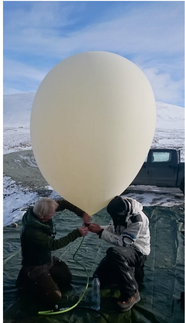
Figure 2. Sealing the first helium filled stratospheric balloon with the help of balloon expert Steven Peterzén
