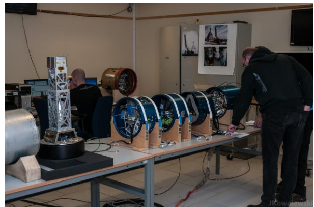
Figure 15. Actual setup of REXUS-21 rocket during interference and bench tests.
