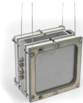
Figure 2. Shear cell furnace used in the XRMON-DIFF 2 module
