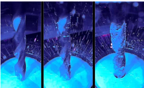
Figure 19. Dust sticking to drill bit in space conditions.
