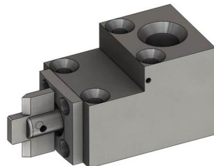
Figure 3 - Bolt cutter used in the separation of the nose cone.
