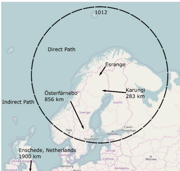
Figure 9. Radius of the direct wave propagation path.
