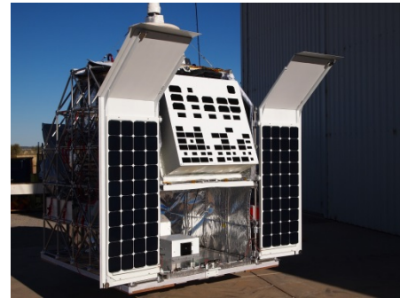
Figure 4. The CARMEN gondola with the pointed-tray of solar cells in the upper middle. (Credit CNES/CNRS - S. Chastanet)
