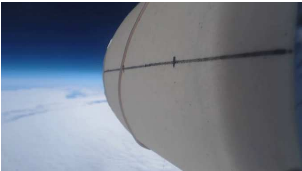
Figure 8. Fully inflated antenna with the helical wound coaxial cable
