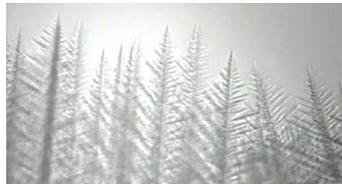
Figure 8.a Columnar dendritic growth
