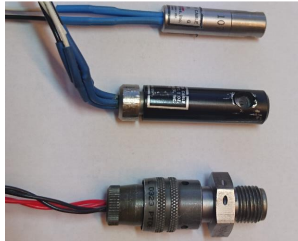
Figure 1 - Horex 2800, 2801, 3702 (top to bottom). The squibs currently in use at Andøya Space Center.
