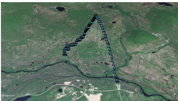
Figure 11. 3D trajectory of the rocket visualized in Google Earth Pro. It should be noted that only 1 out every 100 values was used for plotting this trajectory.
