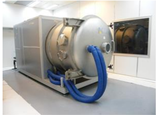
Figure 14. Thermal vacuum chamber
