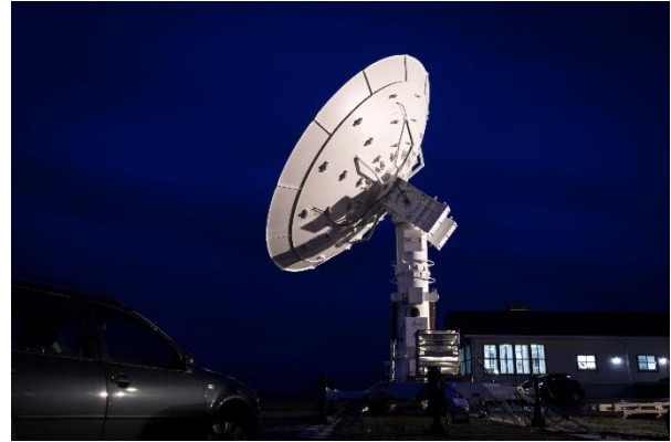
Figur 5 - New 7.3 meter TM antenna at ASC
