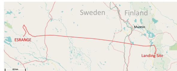
Figure 5. GPS flight path of BEXUS 20 recorded by the CPT-A telemetry unit. Background map credit: OpenStreetMap.
