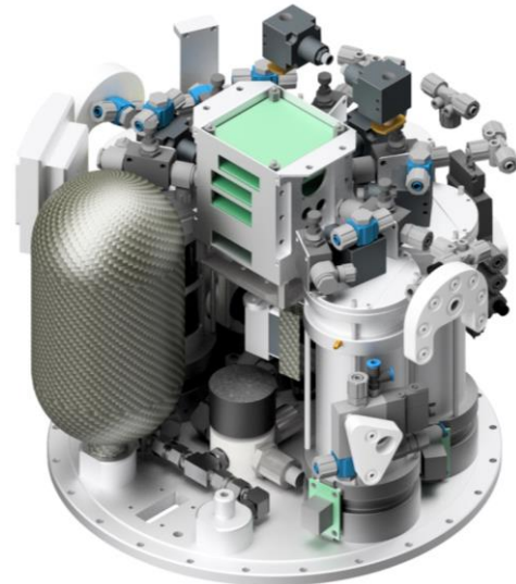
Figure 3. CAD view of UB-FIRE experiment without the module, upper bulkhead, one high pressure bottle and tubing
