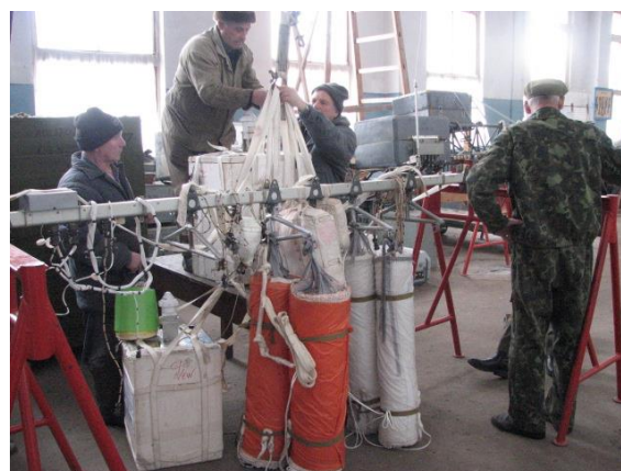
Fig. 5. Installation of a gradiometer on a suspension bracket of a balloon
