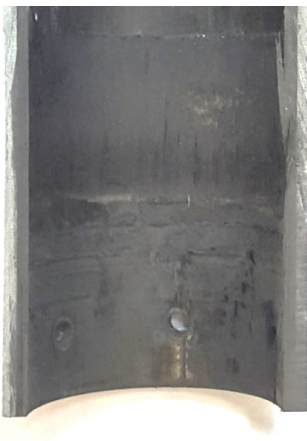
Figure 3: Slight deterioration of casing after test 2
