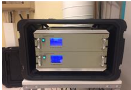
Figure 9 Scientific exciter unit
