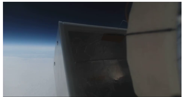
Figure 6. Lid opening after burn-wire activation
