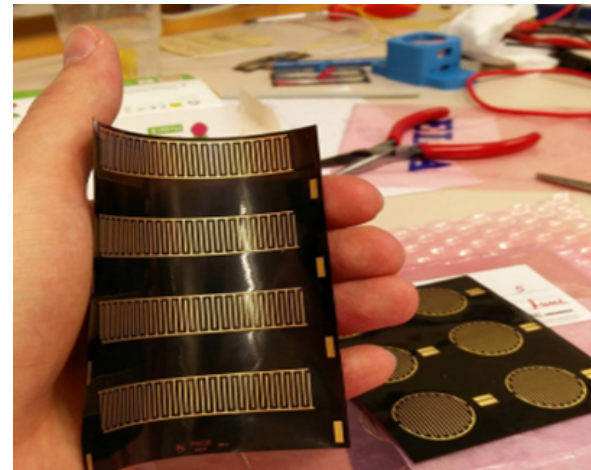
Figure 3. The conductivity sensors were printed on a flexible PCB and glued to the side and bottom of the vessels.
