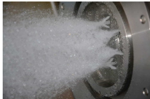
Figure 6: water test of the injecting plate.
