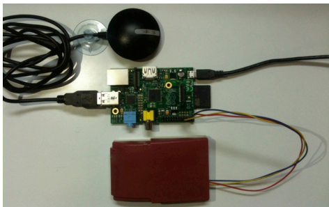
Figure 4 – Prototype - RPi, USB GPS Receiver and BST Detector.
