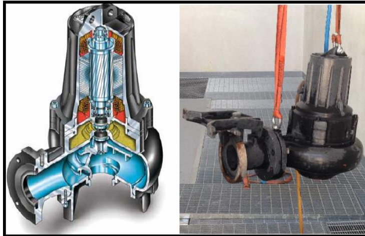
Figure 2 – Grinder pump used in the study
