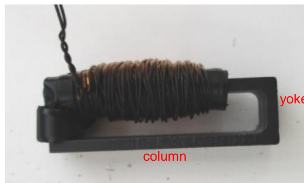
Fig. 16 - SMC sample used to study the effect of magnetic orientation
