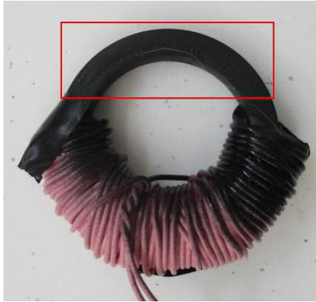
Fig. 1- Surface of the SMC toroid under exam indicated with the red line and matt black painted to avoid reflections
