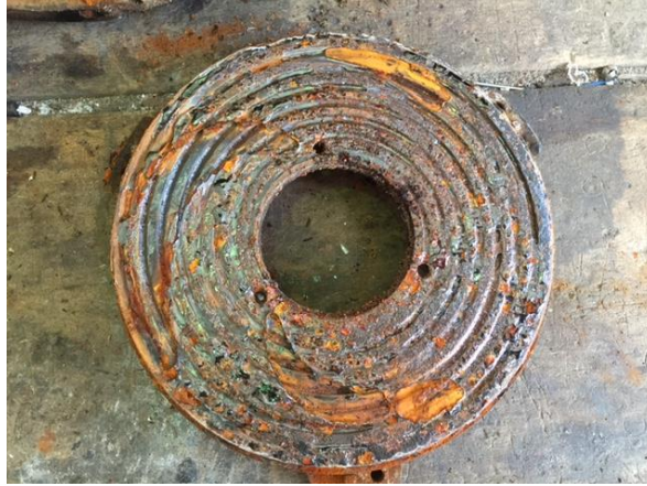
Figure 5 – Inner part of an aged bottom plate
