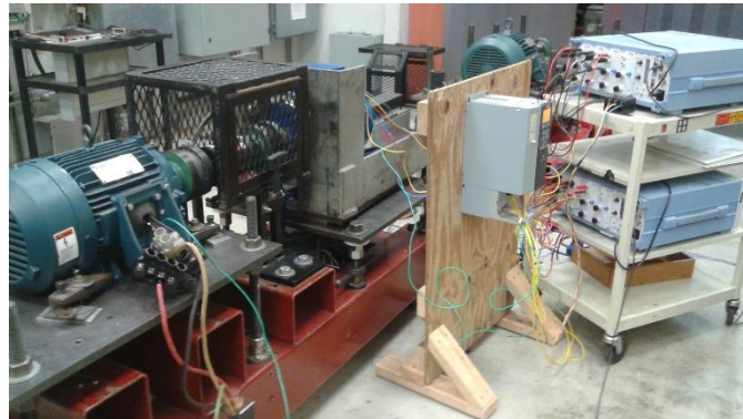
Fig 10: A 7.5hp motor-drive system under test
