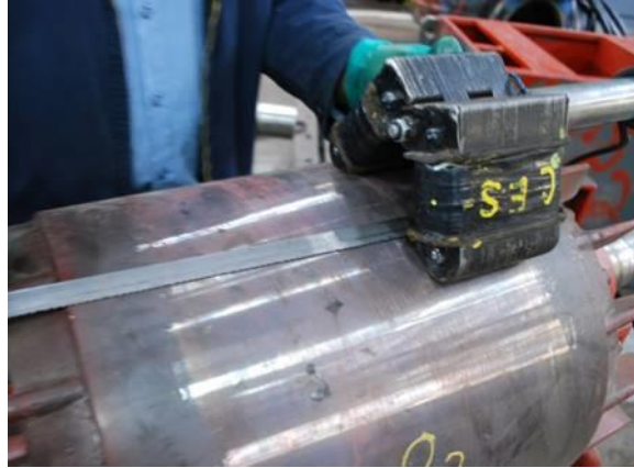
Figure 6: Growler test of a rotor.
