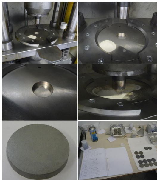
Fig. 7 – Realization of the discoidal samples
