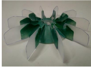
Fig. 6. First prototype of a centrifugal, flexible-blade, cooling fan for a 7.5-kW, 4-pole, self-cooled motor.
