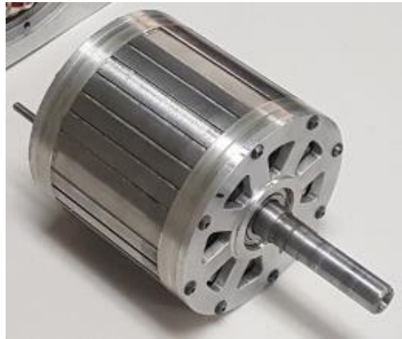
Fig.2. Dual Rotor LSPM Rotor components (a) and assembly (b)
