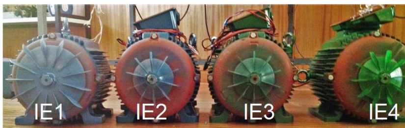
Fig. 1. Cooling fans of 7.5-kW, 4-pole, self-cooled, three-phase induction motors of different efficiency classes (IE1-IE4).
