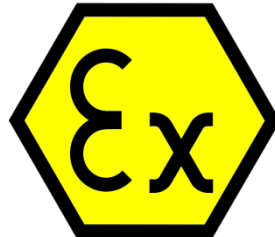
Fig. 14. Mark for ATEX certified electrical equipment for explosive atmospheres (Ex d – Explosion proof multivoltage motors; Ex de – Explosion proof multivoltage motors with increased safety terminal box).
