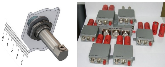
Fig. 1. Electric field probe (left) and surface charge control equipment (right).
