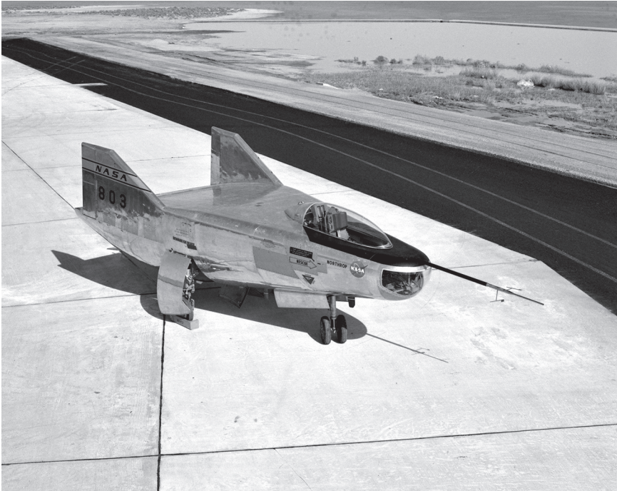
The M2-F2 was the first heavyweight wingless lifting body research aircraft. The half-cone configuration was flown to demonstrate potential characteristics for a future space vehicle capable of entering Earth's atmosphere and landing on a conventional runway. (NASA)
