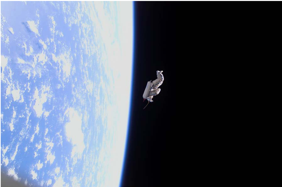
FIGURE 6. SuitSat. Backdropped by the blackness of space and Earth's horizon, a spacesuit-turned-satellite called SuitSat began its orbit around Earth after it was released by the Expedition 12 crewmembers during an EVA on 3 February 2006. SuitSat, a Russian Orlan spacesuit whose utility had expired, was outfitted by the crew with three batteries, internal sensors and a radio transmitter, which faintly transmitted recorded voices of school children to amateur radio operators worldwide. (NASA ISS012-E-16905)
