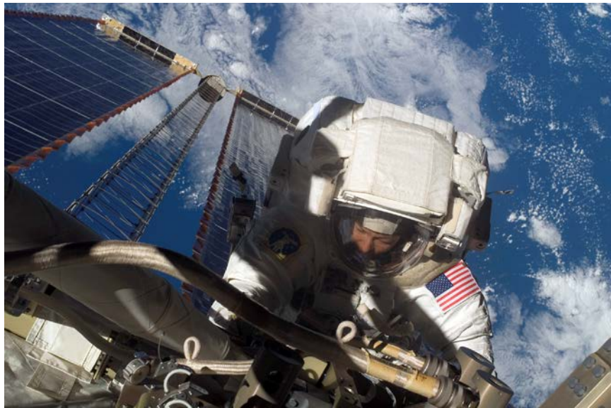
FIGURE 7. ISS 100th Construction Spacewalk. Expedition 16 Commander Peggy Whitson works to re-connect cables on the 1A Beta Gimbal Assembly (BGA) during EVA 13. (NASA ISS016-E-17499)
