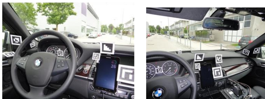
Figure 1. Attachment of the nomadic device and the markers in the test vehicle
