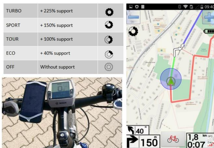
Figure 1. Interface of the EAS prototype (right) with support levels (upper left) and experimental setup at the pedelec (bottom left).
