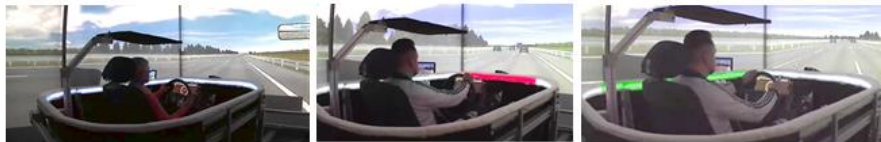
Figure 7. a) Ambient light active, b) Longitudinal warning, c) Lane change recommendation
