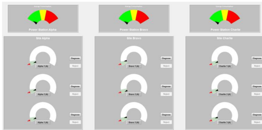
Figure 1. Monitoring screen of ConCenT containing the displays of nine production facilities and three power stations, which are distributed over three locations
