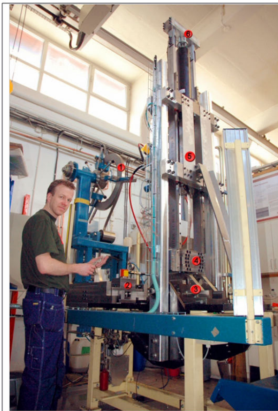
Fig 1a BUT machine. (1) coil, (2) grip for brake force, (3) tool holder, (4) grip for pulling
