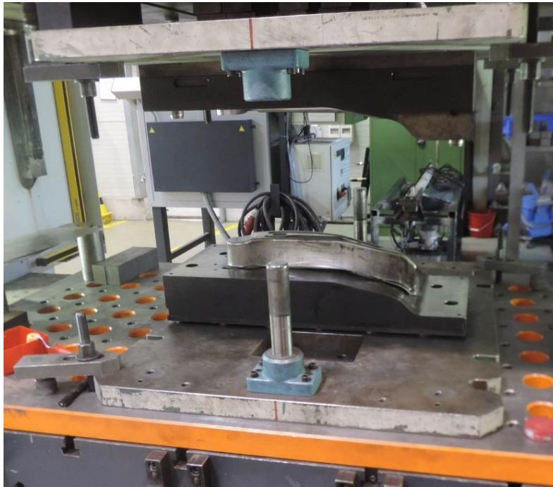
Figure 2.9.10: Lower part of the prototype tool installed in a tryout press at SZMF
