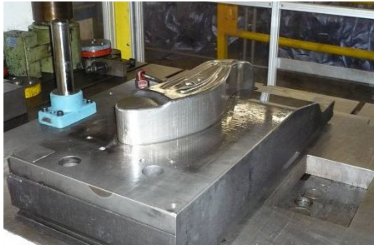
Figure 2.9.3: Lower part of the chosen prototype tool
