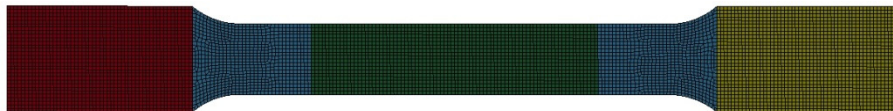
Figure 2.7.14: Numerical model for the simulation of the tensile test. Discretization of the specimen with shell elements, an element size of 1 mm was used.
