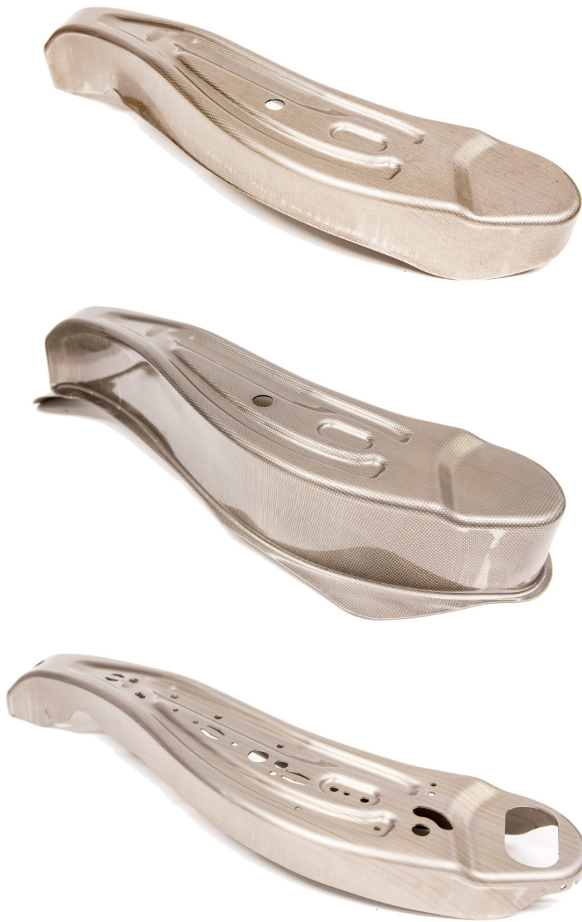
Figure 2.9.13: Prototype component made of TWIP-steel. Top: blank type 1, centre: blank type 2, bottom: after laser cutting
