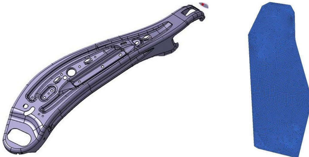
Figure 2.9.2: CAD model of the backrest sidemember (left) and blank dimensions 272 mm x 679.9 mm x 1,5 mm (right)
