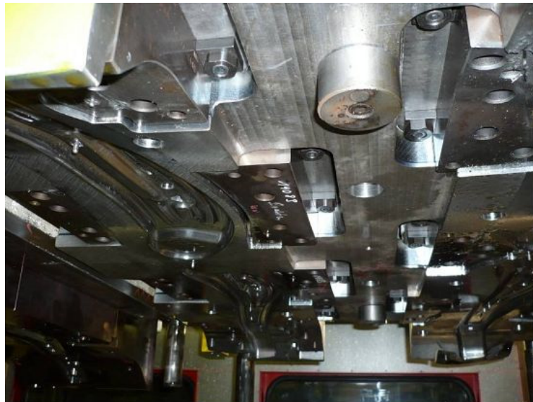
Figure 2.9.4: Upper part of the chosen serial tool
