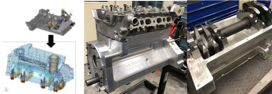
Fig. 1. LSE billet block, crankshaft and connecting rod. Cylinder head is equipped with a fully flexible valve actuation system by Sturman Industries. Engine was built for single cylinder operation. Custom crankshaft was built with two counterweights for overall engine balance.
