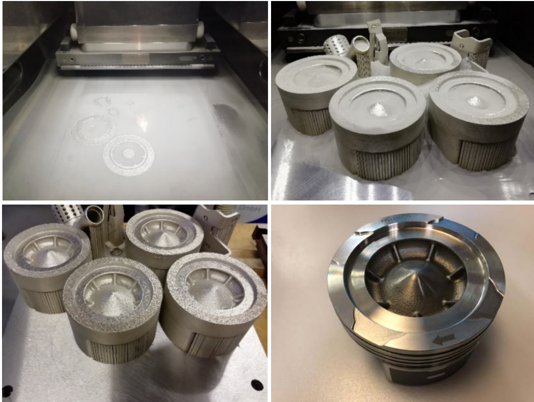
Fig. 8. Set of views of the AM pistons during the printing process: from the first layers to the final rough pieces. The last picture shows the final part and bowl surface quality after the full machining.
