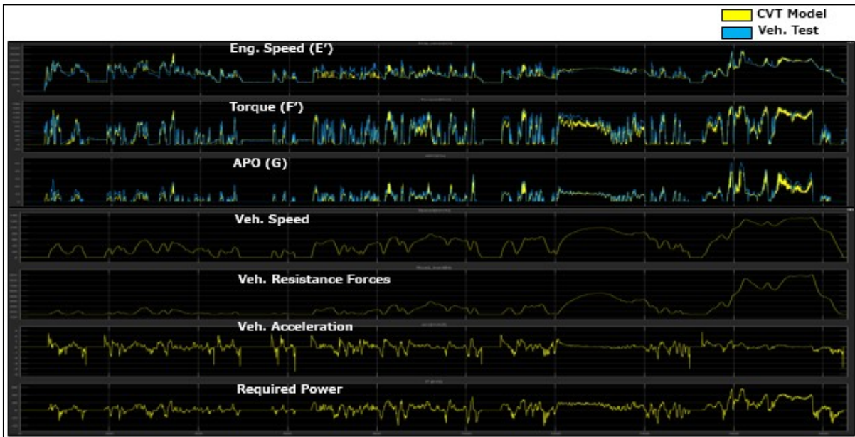
Fig. 5. CVT model behaviour for WLTC
