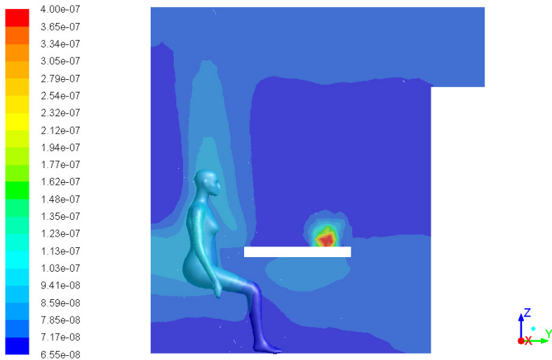
Fig. 7. Mass fraction of pollutant UDS1 [kg/kg] in a vertical mid-plane through the mannequin
