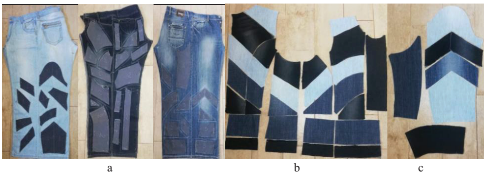
Fig. 5. Laying the production patterns on the jeans and cutting the details of the jacket
