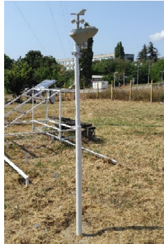
Fig. 5. Meteorological station located in the experimental field of Technical University – Varna
