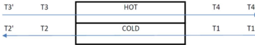
Figure 1. Basic scheme of counterflow heat exchanger.
