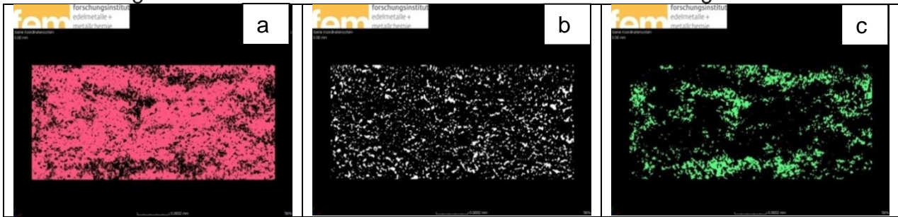
Fig. 5. FIB cuts ( 15 \times 15 \times 30 \text{ nm}^3 ) of in-house fabricated substrate, evaluated with VG-Software. a) graphite b) pores and c) PTFE.
