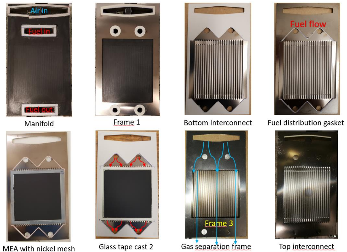
Figure 2: Sequence of a single cell stack assembly.
