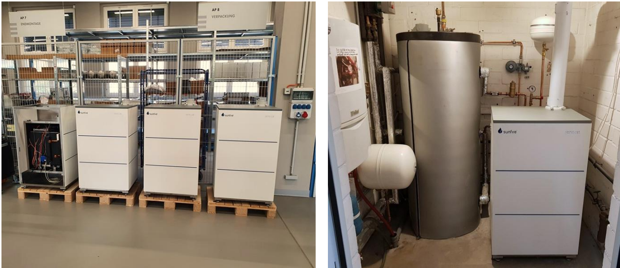
Figure 5. Small scale series production at Sunfire Fuel Cells and first installed customer systems in operation
