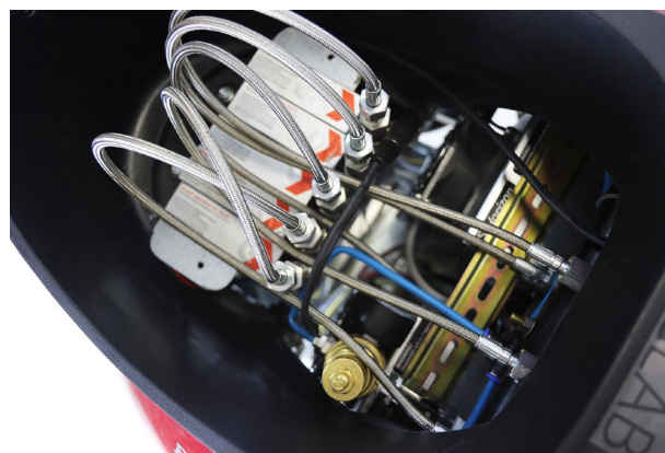
Fig. 6. Main MH tank, composed by five cartridges, and fuel cell system, on the scooter prototype.
