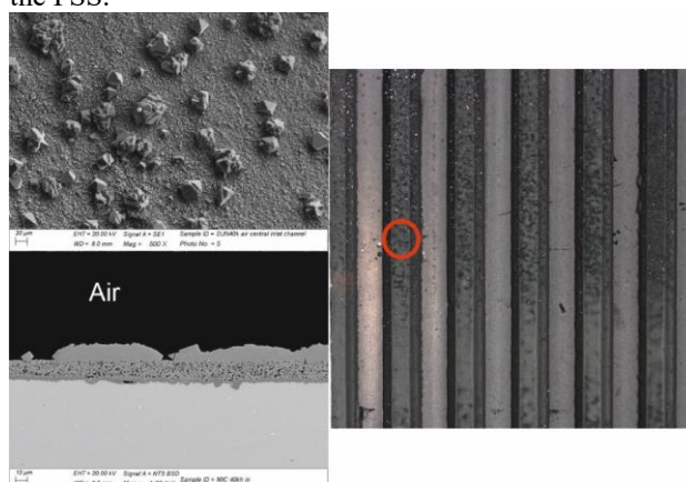
Fig. 4. Air side, central area inside a channel with large spinel crystals containing Mn, Co, Cr, Fe on top of the MCO coating. Details are visible on the cross section image
