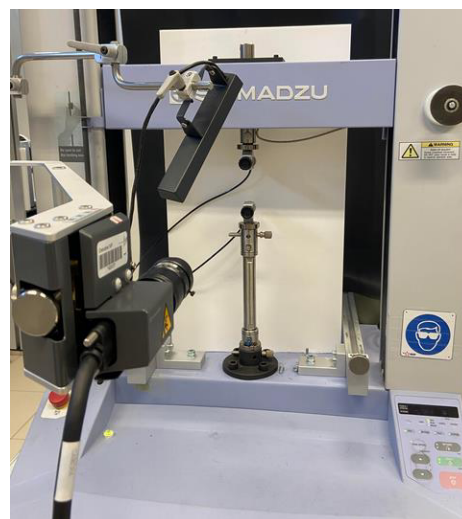
Figure 2. Tensile test bench equipped with a video extensometer
