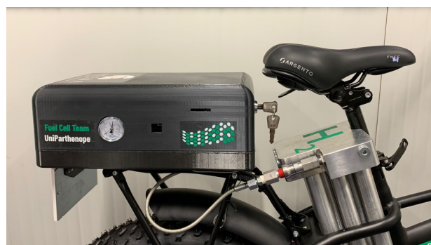
Fig. 5. Casing of the HyBike power unit.
