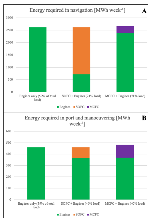
Fig. 6: Total daily energy required by the LNG fuelled ship during navigation (A) and during manoeuvring and port activities using traditional engines only, and the engines integrated with an SOFC or an MCFC system.
