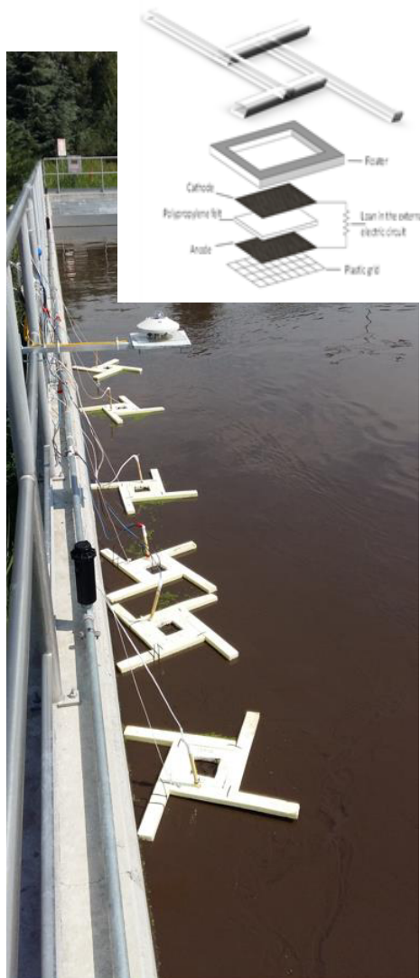
Figure 1. Planar MFCs floating in the anoxic tank of the wastewater plant during the test. The schematic of MFC components is reported right on the top.
