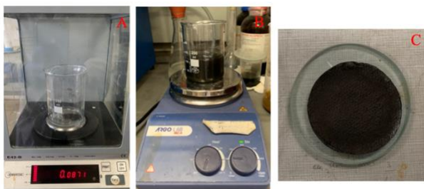
Fig. 1. Protocol to produce the multicomposite Cu@/HAP/C.
