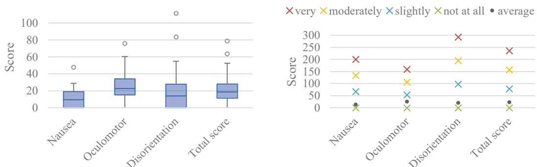
Figure A – Left: SSQ profile of the audiovisual system in the test (original score); Right: overview of SSQ subscale and corresponding verbal ticks.
