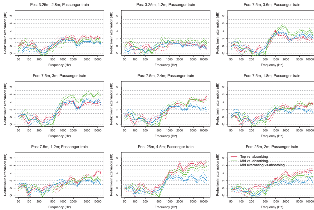
Figure 3: Measured reduction in attenuation for passenger train. Different settings are color coded. Dashed lines show the standard error of the mean. Positive values indicate a reduction in attenuation when using reflecting panels compared to a fully absorbing barrier.
