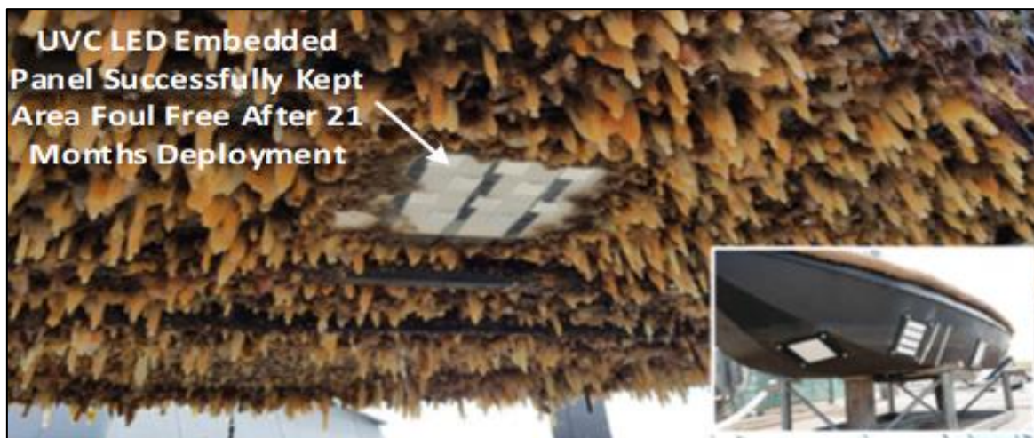
Fig.1 - Demonstration of UV-C LED Fouling Prevention, Jongerijs et al. (2018)
