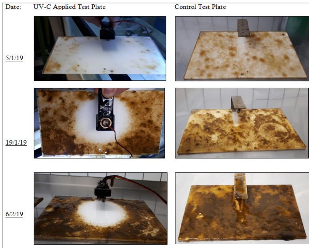
Fig.6: Test Plate Growth Record with Reduced Exposure Time
