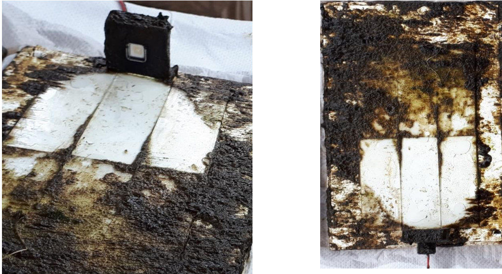
Fig.7: Effective Antifouling Distance of UV-C LED
