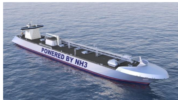
Fig.5: Ammonia-fuelled conceptual ship design for a tanker, De Vries (2019)
