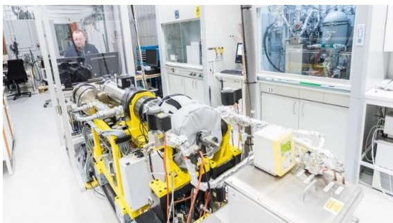
Fig.4: Dual-fuel diesel for ammonia on test bed, source: Wärtsilä
