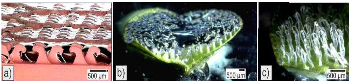
Fig.1: Biomimetic microstructure (a) and leaf of the Salvinia plant (b) with micro-structured hydrophobic hairs (c)
