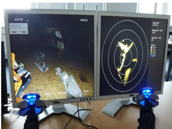
Fig.6: PC-based VR training for underwater vehicle handling
