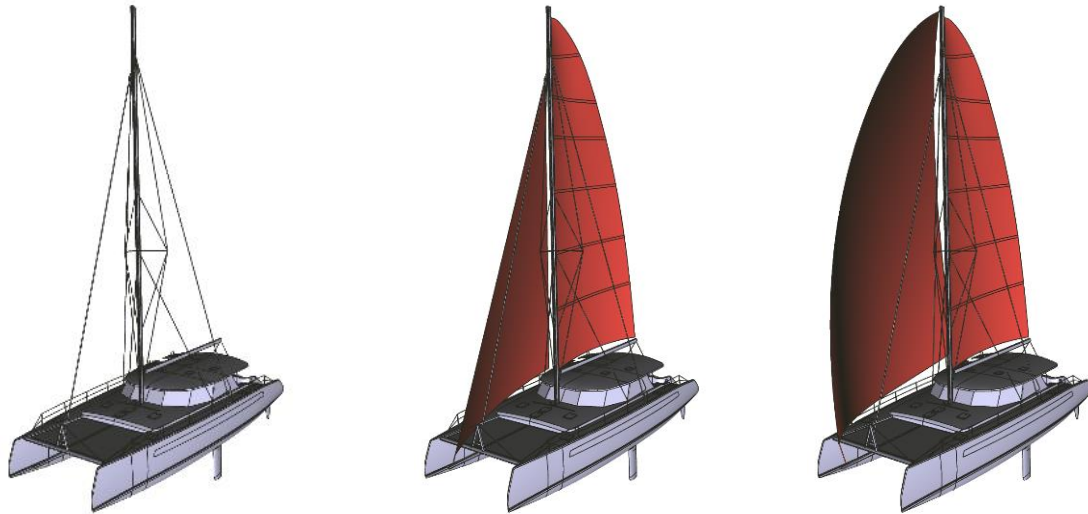
Fig.4: CAT CAD geometry and two sail configurations: main and genoa (mid) and main and spinnaker (right)
