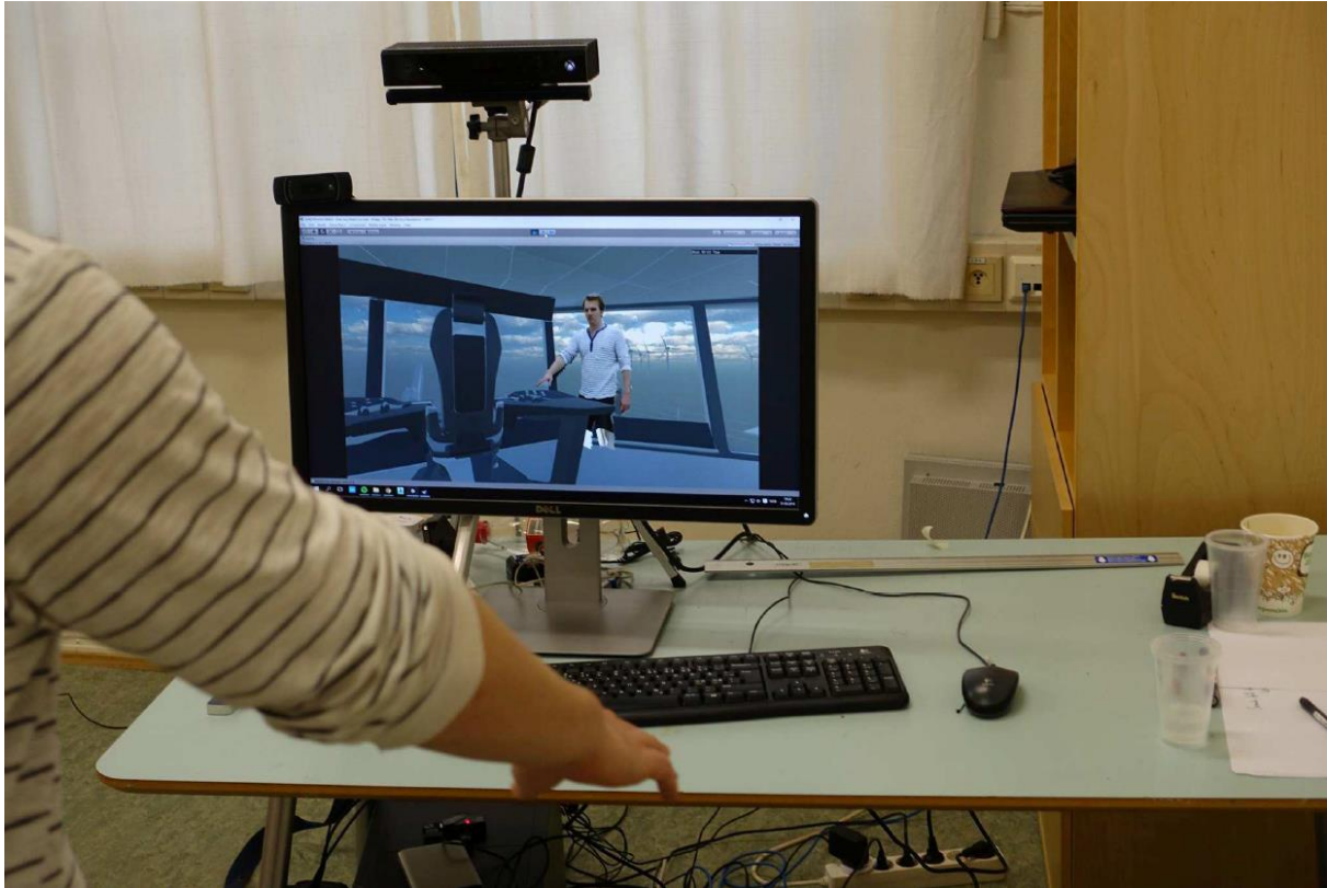
Fig.20: 3D scanner and view of VR view with avatar on bridge
