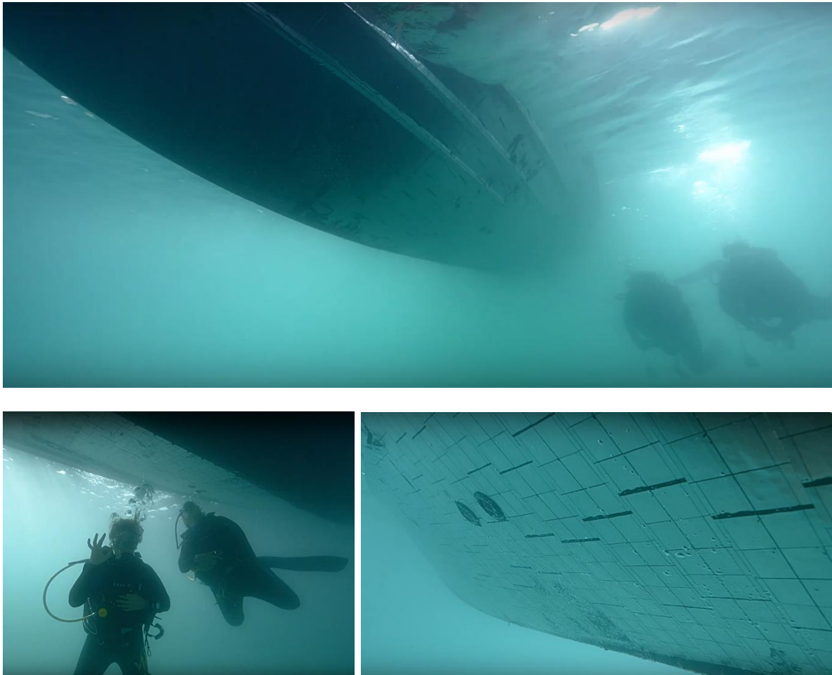
Fig.5: Underwater shots after a first test run. The air layer is clearly visible. The dark stripes are unstructured areas of the film.
