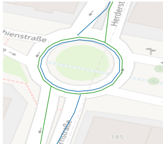
Figure 4: Faulty detection of two driving directions due to a wrongly assigned oneway attribute in OSM
