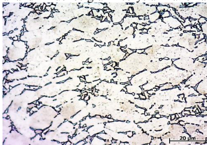
Fig.1 As received microstructure of titanium alloy Ti6Al4V in annealed condition Fig. 2. Heat treatment (solution treatment and annealing)
