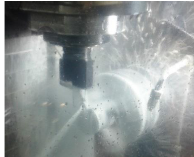
Fig. 6 On machine high pressure coolant set up for rake face of the tool
