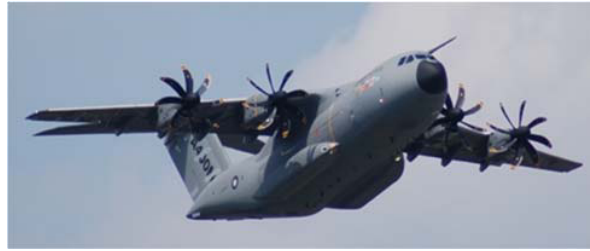
Fig. 1. Airbus A400M - The wings (over 20 m long and 4 m wide) consist mainly of CFRP
