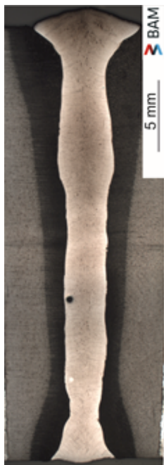
Fig. 6. Cross section of single-pass weld
