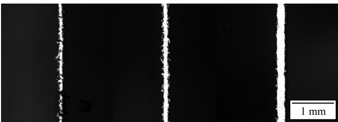
Fig. 3. Cross sections of different wall structures, left too thin (65.2 \mu\text{m} ), middle desirable (115.2 \mu\text{m} ), right too thick (203.1 \mu\text{m} )
