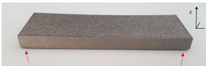
Fig. 9. Test sample C2, building direction along z-axis.
