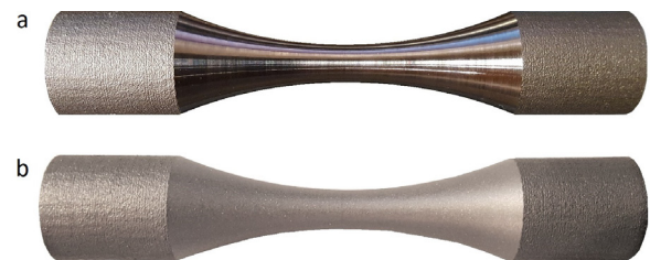
Fig. 4. (a) machine finished; (b) blasted finished
