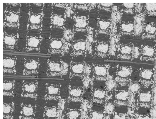
Fig 8. BSE image of fractured surfaces after lap shear tests. General view.
