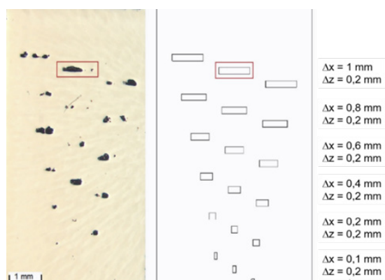
Fig. 2. Comparison of a section of the prepared test specimen (left side) with the volumetric cavities placed in the CAD model (right side).
