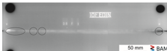
Fig. 7. X-ray image of a single-pass weld seam with defects (black circled)
