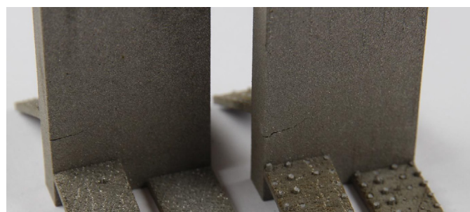
Fig. 2. Benchmark part no. 1 (left: block support, right: pin support) after support removal.
