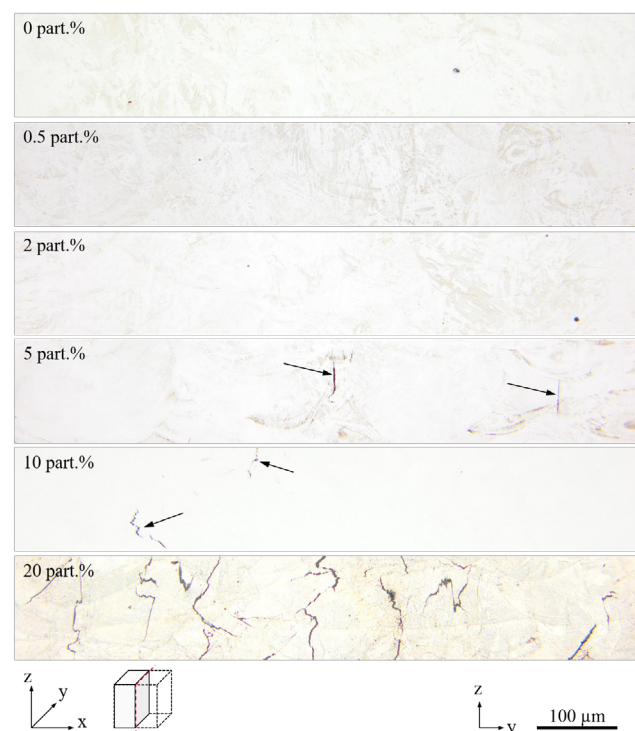
Fig. 1. Light microscopy images of etched cross-sections of the y-z-plane of cubic specimens, where z indicates the build direction and arrows mark cracks at 5 and 10 part.%.
