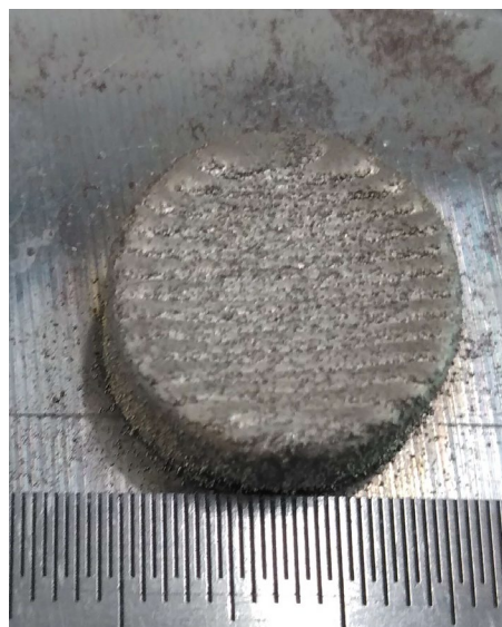
Fig. 1. LPBF of the NiCrBSi alloy (top view)
