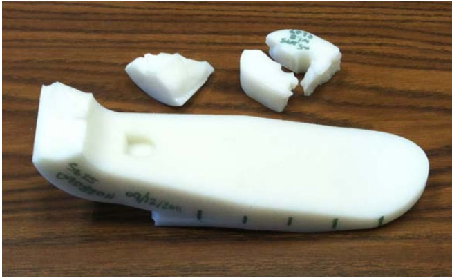
Fig. 2. PBF-LB/P polyamide 11 prosthetic foot which shattered a low load [3]. The green marks on the main piece are spaced at 25 mm.
